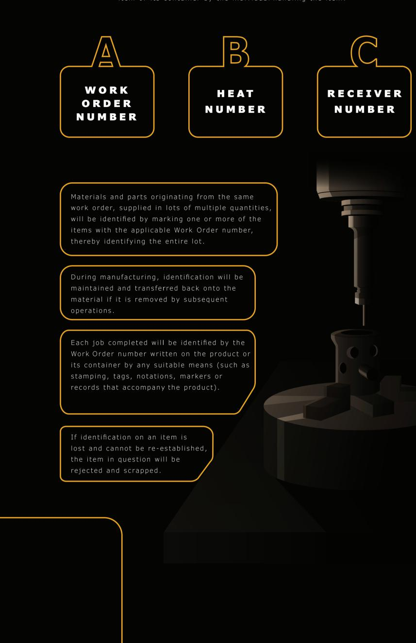
Identification for manufactured parts will be performed by the individual starting the job by recording the appropriate information as required on the applicable Work Order and recording the Work Order number on the
